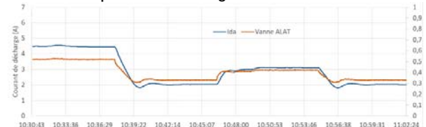
Figure 15 : Downstream pressure regulation for 3 bar upstream pressure
