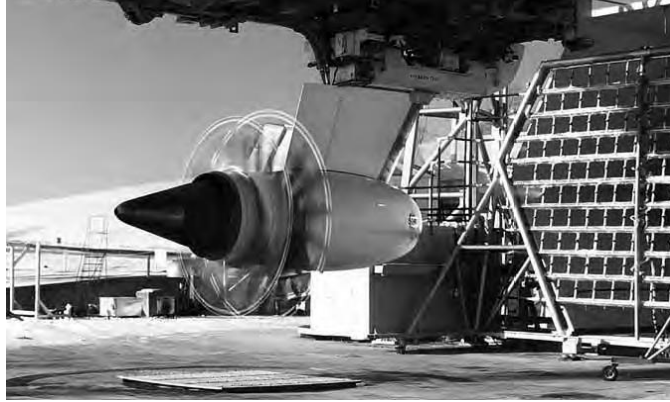
Figure 2. GE36 “Unducted Fan”: a Rear-Mounted “Pusher” CROR Configuration. 5
