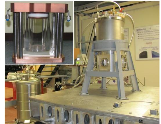
Experimental detection of wall angles and free surface topology (VKI)
