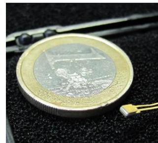
Cryogenic temperature transducer (VKI)
