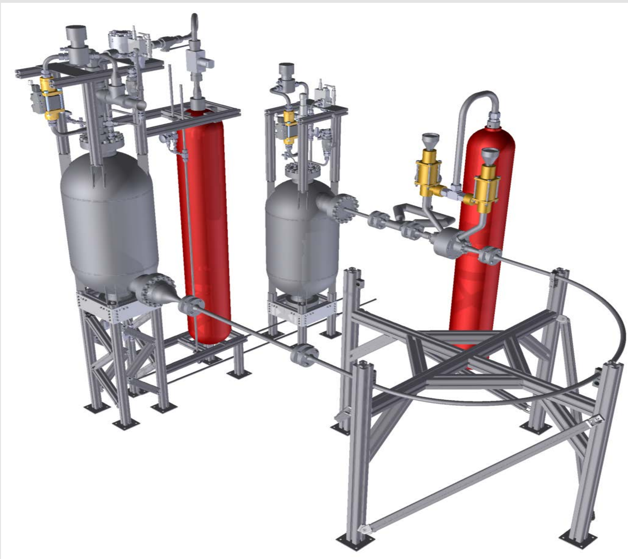
Fluid Transient Test Facility M3.5 at DLR for investigation of water hammer and priming in LRE feedline. Test fluids are water, ethanol, LN2 and LOx
