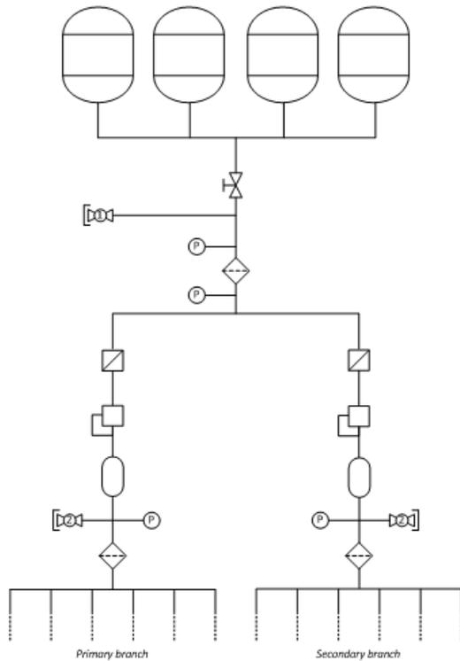
Figure 8 – Euclid MPFA schematics (credit: OHB Sweden)
