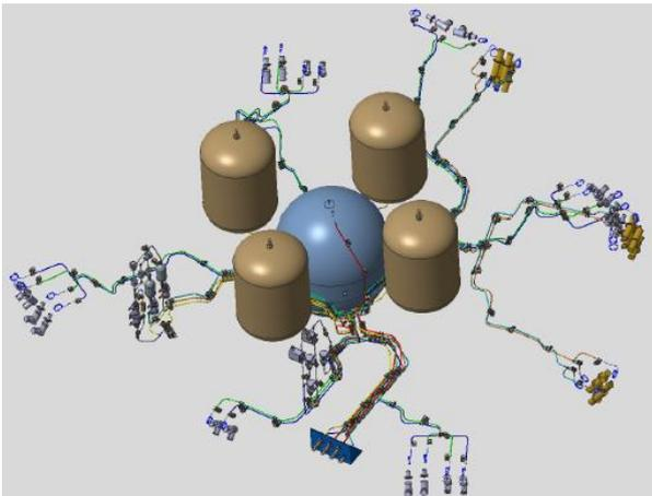
*Figure 10 – Euclid RCS and MPFA tube routing from the tanks to the thrusters (credit: OHB Sweden)*
