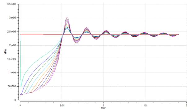
Figure 7 – Pressure in the propellant lines in function of time during Euclid RCS priming (credit: OHB Sweden)
