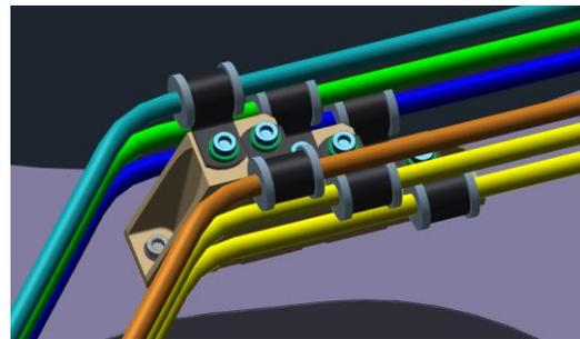
*Figure 11 – Tube standoff supporting both RCS and MPFA tubes (credit: OHB Sweden)*
