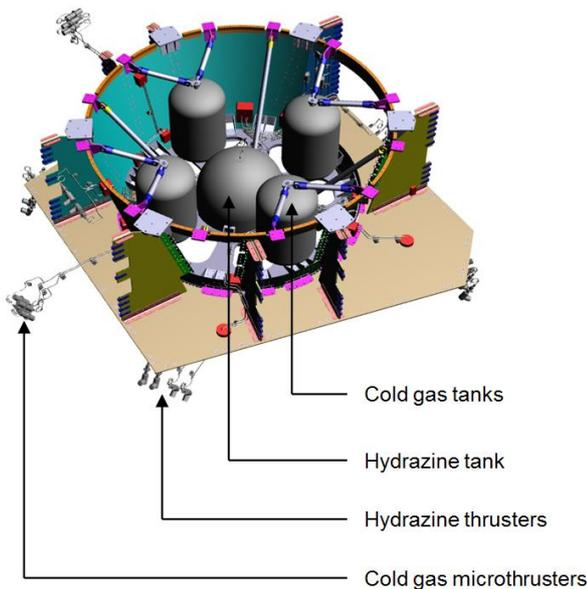
Figure 4 – Open view of the Euclid Service Module illustrating the location of the four cold gas tanks and of the Hydrazine tank (credit: OHB Sweden / TASI)
