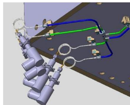
*Figure 12 – RCS thruster pairs and associated alignment spirals (credit: OHB Sweden)*
