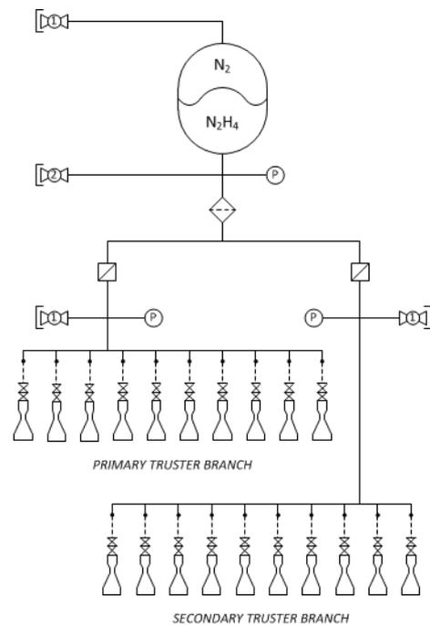
Figure 5 – Euclid RCS schematics (credit: OHB Sweden)
