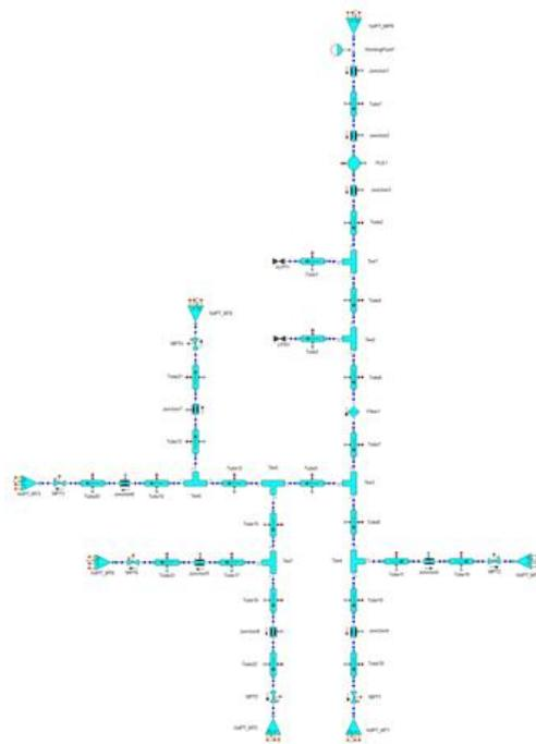
Figure 9 – EcosimPro schematics of the Euclid MPFA, downstream the pressure regulator in one branch (credit: OHB Sweden)
