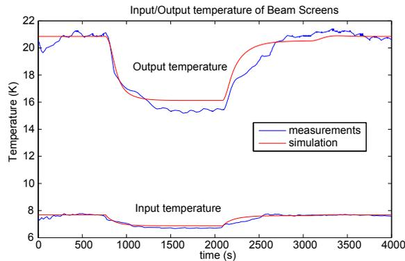
Figure 6: Open loop simulation compared to experiment performed on the LHC String 2
