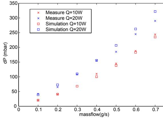
Figure 5: Experimental and simulated pressure drop in steady-state for different heat loads.
