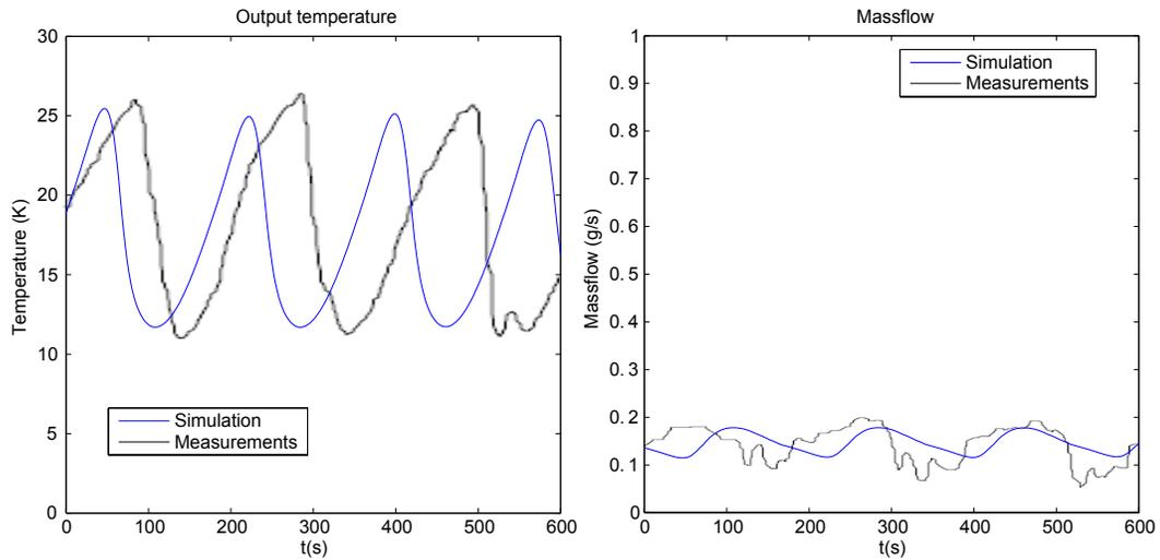
Figure 8: Thermally induced flow oscillations reproduced in simulations and compared with experimental data for a heat load of 10 W and an inlet temperature of 5 K
