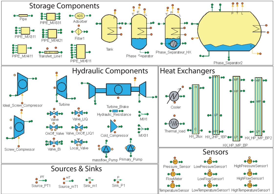
Figure 1: Different cryogenic equipments modeled in the Ecosimpro cryogenic library
