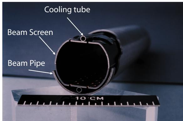
Figure 2: LHC beam screen cooled by its two small cooling tubes
