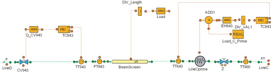
Figure 4: LHC beam screen cooling schematic in EcosimPro
