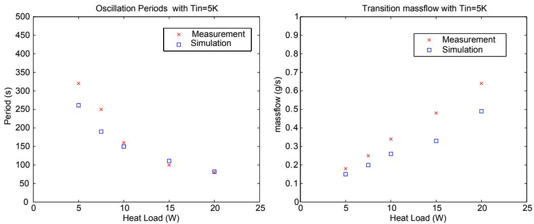
Figure 9: Oscillation periods and mass flows at the transition regime for an inlet temperature of 5 K
