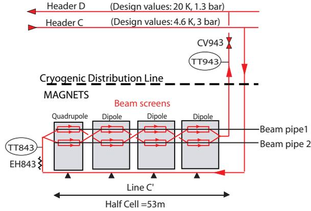
Figure 3: LHC beam screen cooling scheme
