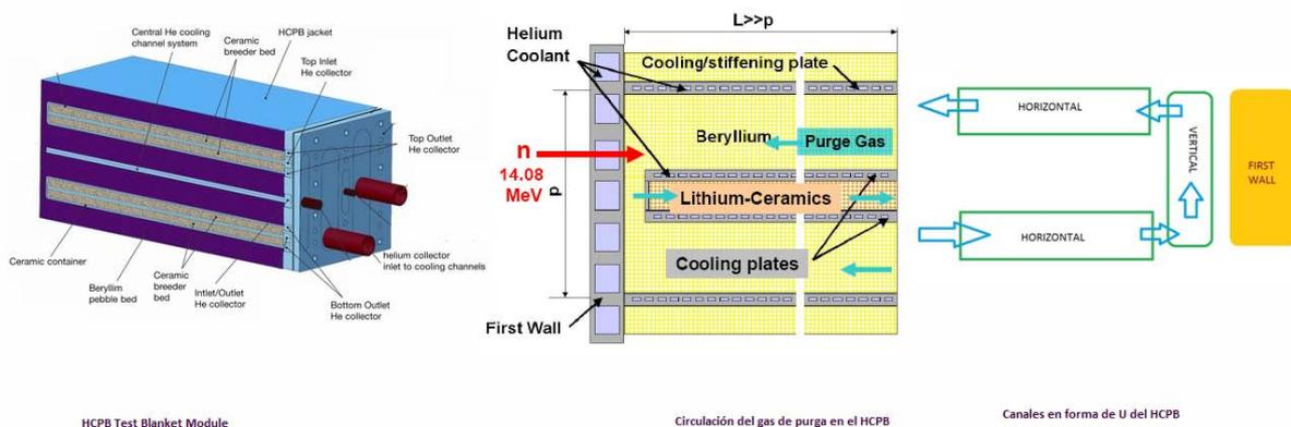
**Figure 3. HCPB Test Blanket Module**
