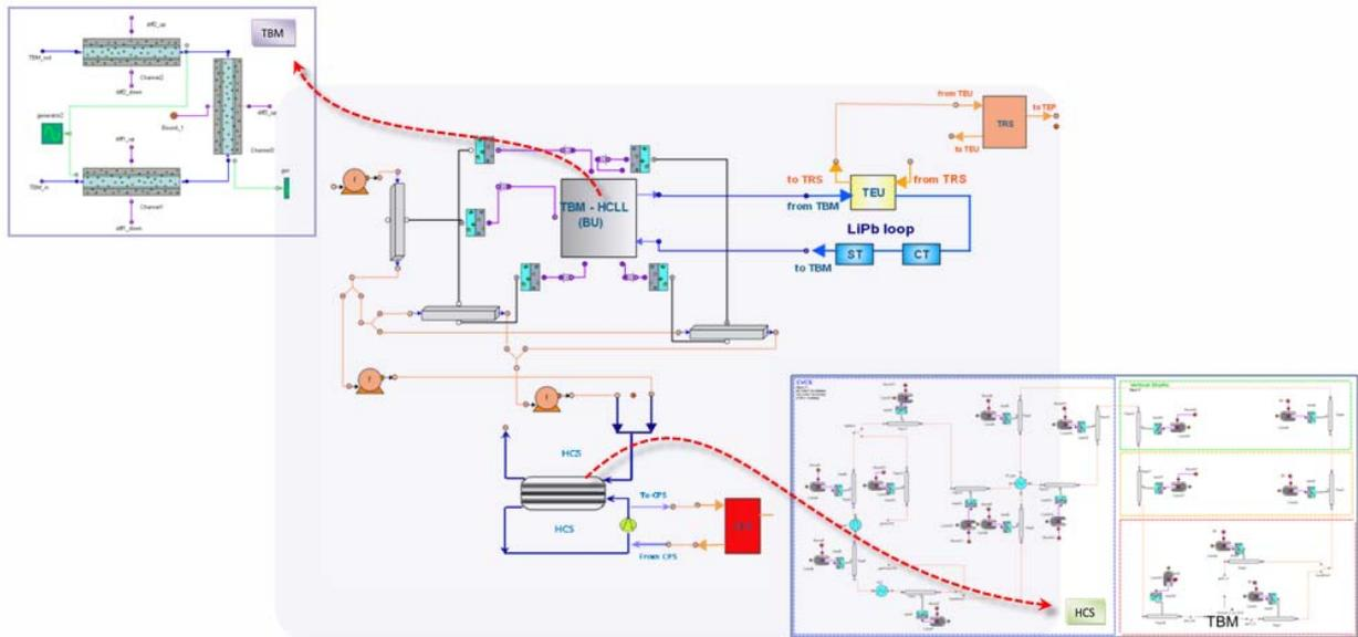
**Figure 5. EcosimPro schematic diagram of the TBS-HCLL system**
