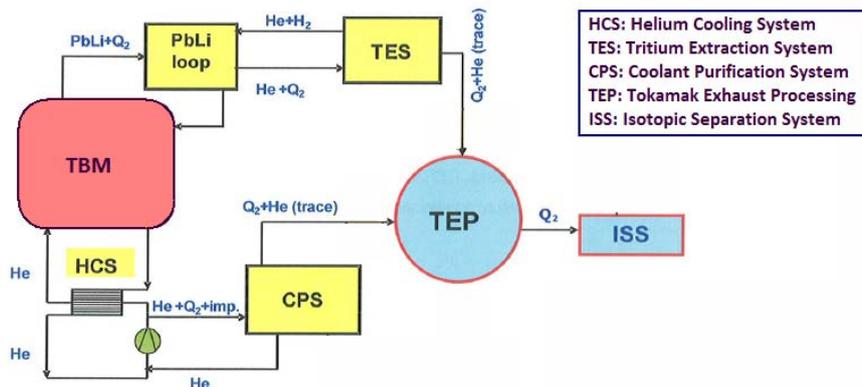
**Figure 1. Diagram of HCLL-TBS. For the HCPB-TBS system the diagram is similar, eliminating the LiPb loop.**
