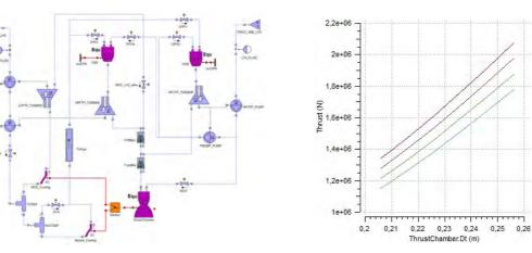
Steady model and parametric analysis of the Space Shuttle Main Engine
