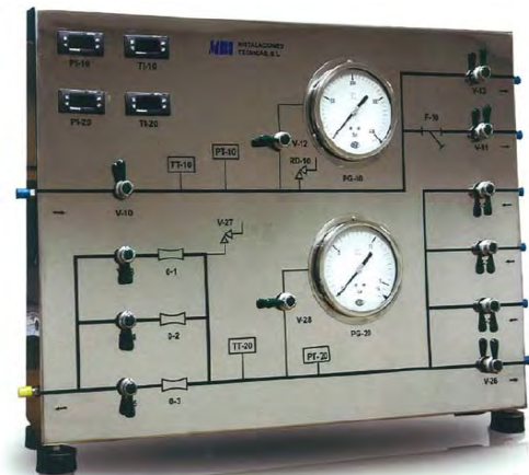
Figure 6: Picture of the Pressurization Panel (PP)
