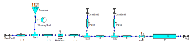
Figure 12. Schematic view of the experimental set-up under EcosimPro.
