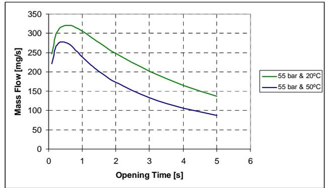
**Figure 9: Average mass flow supplied by PSA at 55 bar in HPN**
