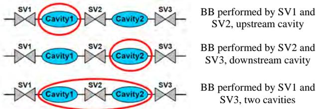
**Figure 2: PSA's BB valves: Upstream Cavity BB, Downstream Cavity BB, Double Cavity BB**
