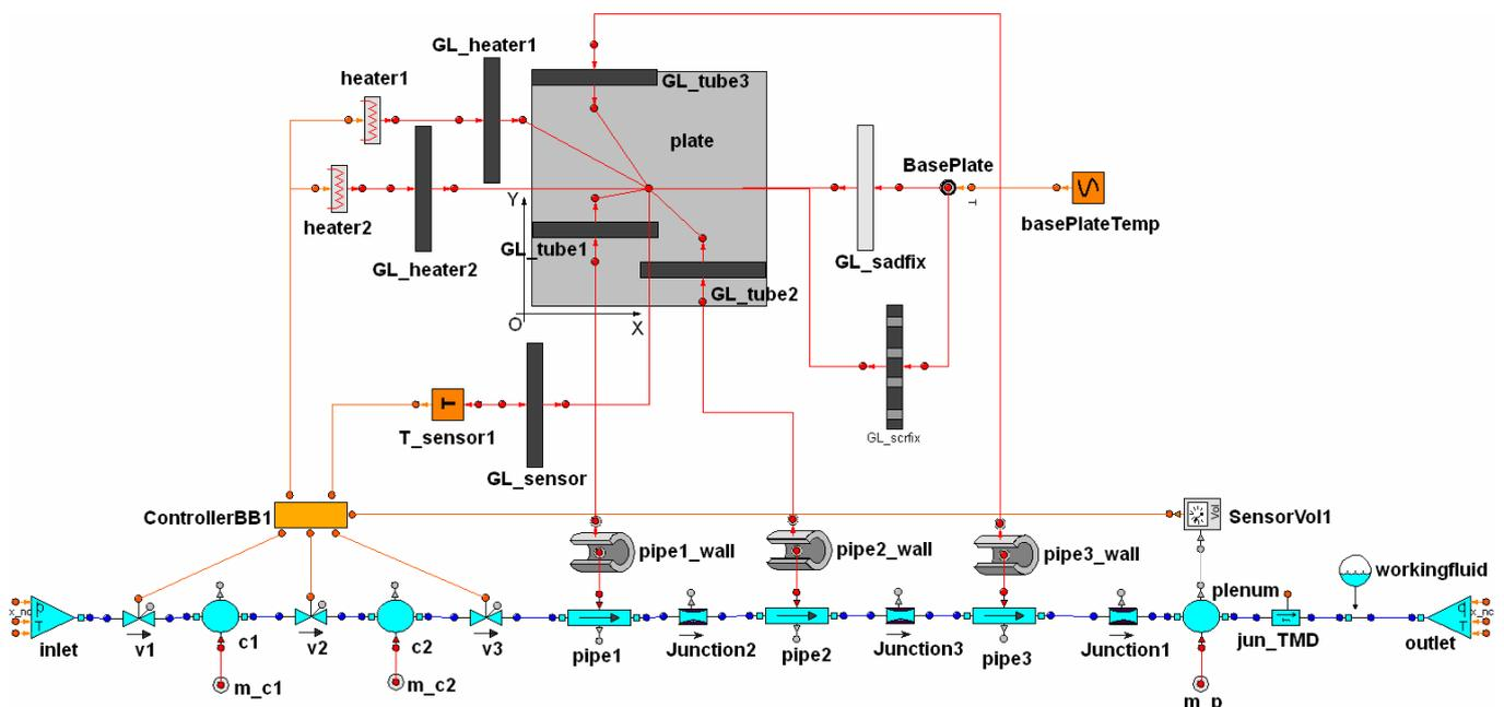
**Figure 7: Schematics of the EcosimPro simulation model of the SGEO PSA**
