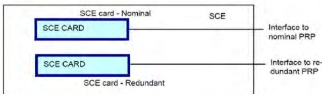
**Figure 3: PSA SCE schematic block diagram**
