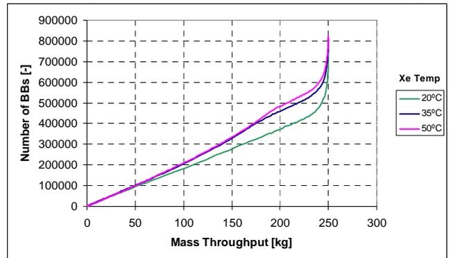
**Figure 11: Number of Bang-Bang Activations vs. Mass Throughput**
