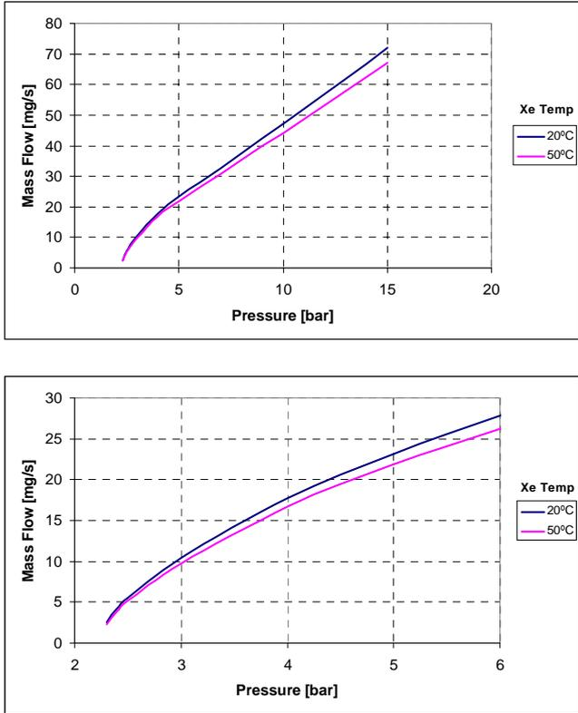
**Figure 8: Maximum mass flow at different HPN conditions at EOL**
