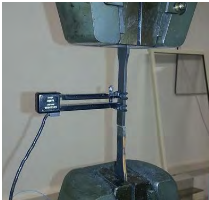
Figure 24 – Specimen of brazed joint Inconel/copper alloy under stress test
