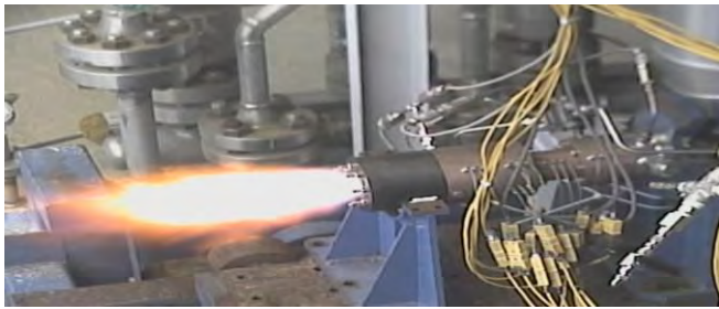
Figure 42 – Firing of the igniter integrated on the chamber
