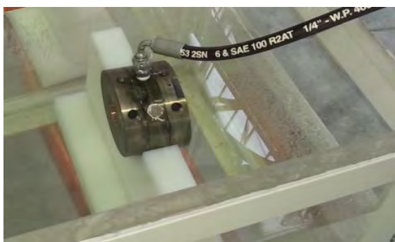
Figure 25 – Cooling disk module under proof/burst testing
