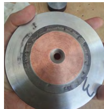
Figure 23 – Specimen of brazed joint Inconel/copper alloy
