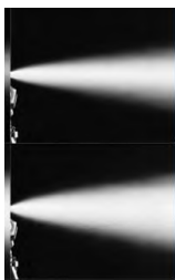
Figure 30 - Jet images captured by camera with and without orifice
