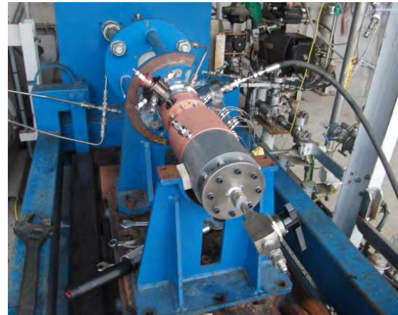
Figure 40 - Heat sink chamber on FAST2 test bench under proof test
