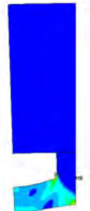
Figure 38 Equivalent plastic strain contour plot after 5 cycles, chamber section
