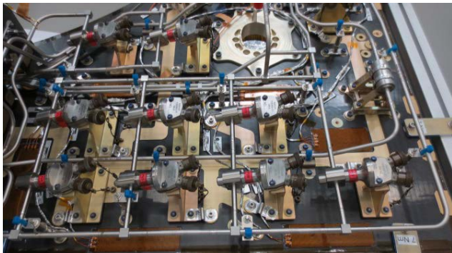
Figure 3-4: Pyrovalve-ladder on ExoMars TGO Pressure Control Assembly (PCA)
