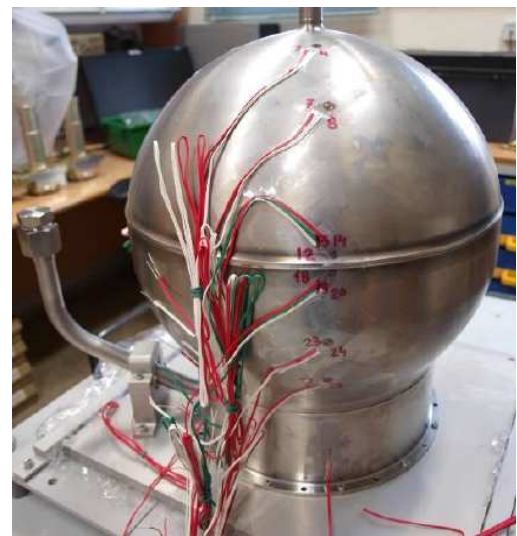
Figure 8 – Propellant Tank under test
