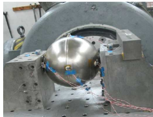
Figure 8 – Helium Tank under test
