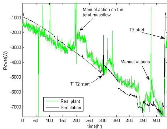
Fig. 10 Energy balance of the overall system
