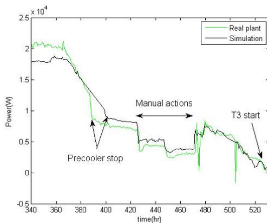
Fig. 11 Energy balance of the Coil Cryogenic System
