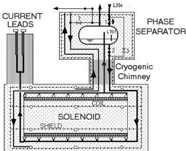
Fig. 2 The Coil Cryogenic System
