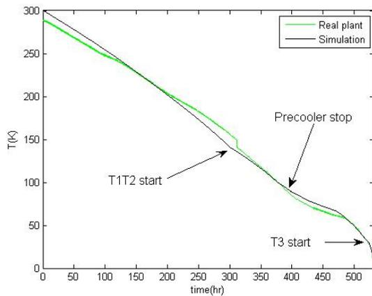
Fig. 5 Magnet temperature
