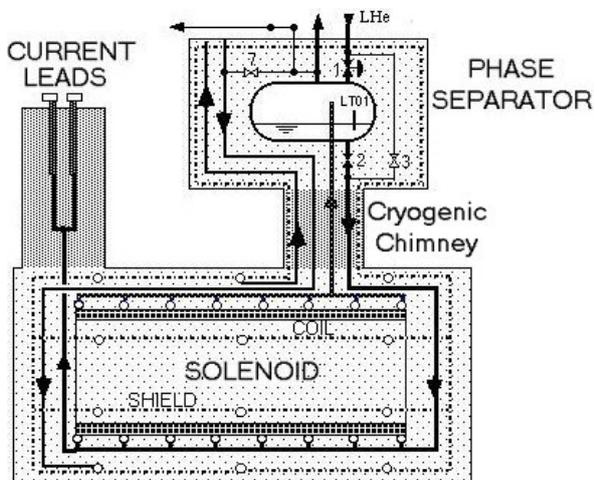
Fig. 2 The Coil Cryogenic System
