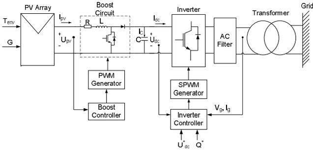
Figure 1.- Block diagram of a grid connected two stage PV System
