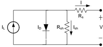
Figure 2.- Circuit diagram of a solar cell
