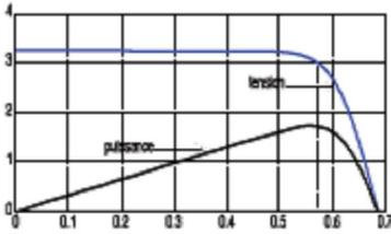
Figure 3.- I-V and P-V photovoltaic array characteristic [1]
