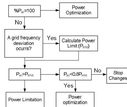
Figure 12.- The flow chart of Switch Cross Coupling
