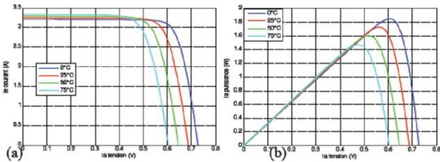
Figure 5.- Temperature dependence of the P-V characteristics at constant irradiation  $E=1000\text{ w}/\text{m}^2$ . (a) I-V curves, (b) P-V curves [1]
