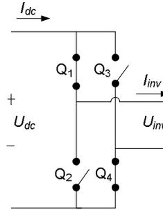
Figure 6.- Structure of the single phase voltage source converter
