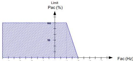
Figure 11.- Frequency Shift Power Control
