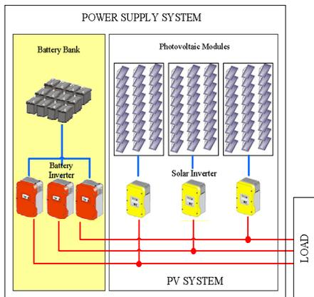
Figure 10.- Block diagram of a stand-alone grid
