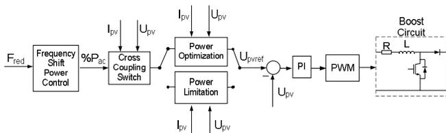
Figure 9.- Boost Controller Model
