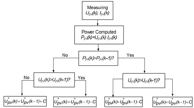
Figure 5.- The flow chart of P&O method [3]
