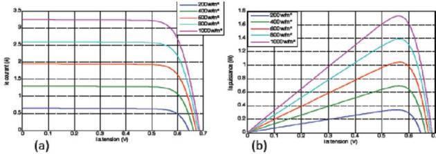
Figure 4.- Irradiation influence on PV array characteristics at constant temperature  $T=25^\circ\text{C}$ . (a) I-V curves, (b) P-V curves [1]
