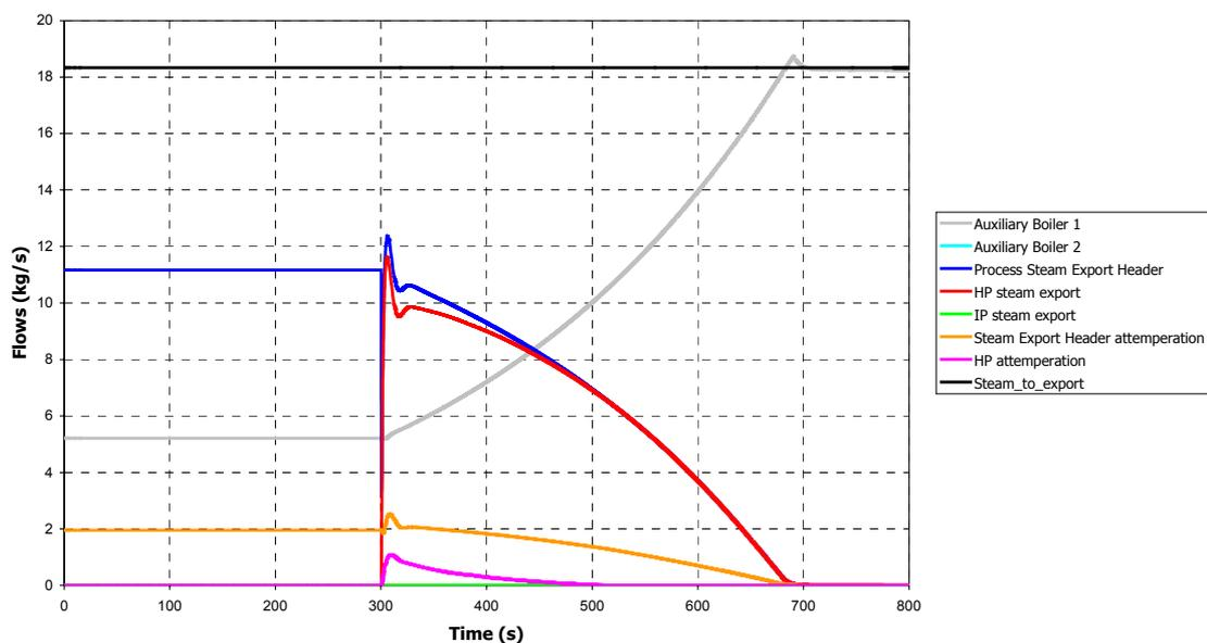
startup, the residual heat from the heat recovery steam generator is used to continue generating steam at a progressively lower pressure and temperature. The evolution of this pressure and temperature is a datum supplied by the boiler manufacturer.
