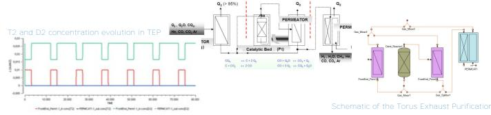
The graph shows how, in a pulsed feed stream containing T2 and D2, the concentration at the outlet of these species is much lower due to the existing extraction systems by permeation in the TEP.
