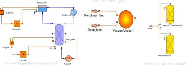
Torus Exhaust Purification (TEP) System: extraction of tritium from the reactor outlet gases
