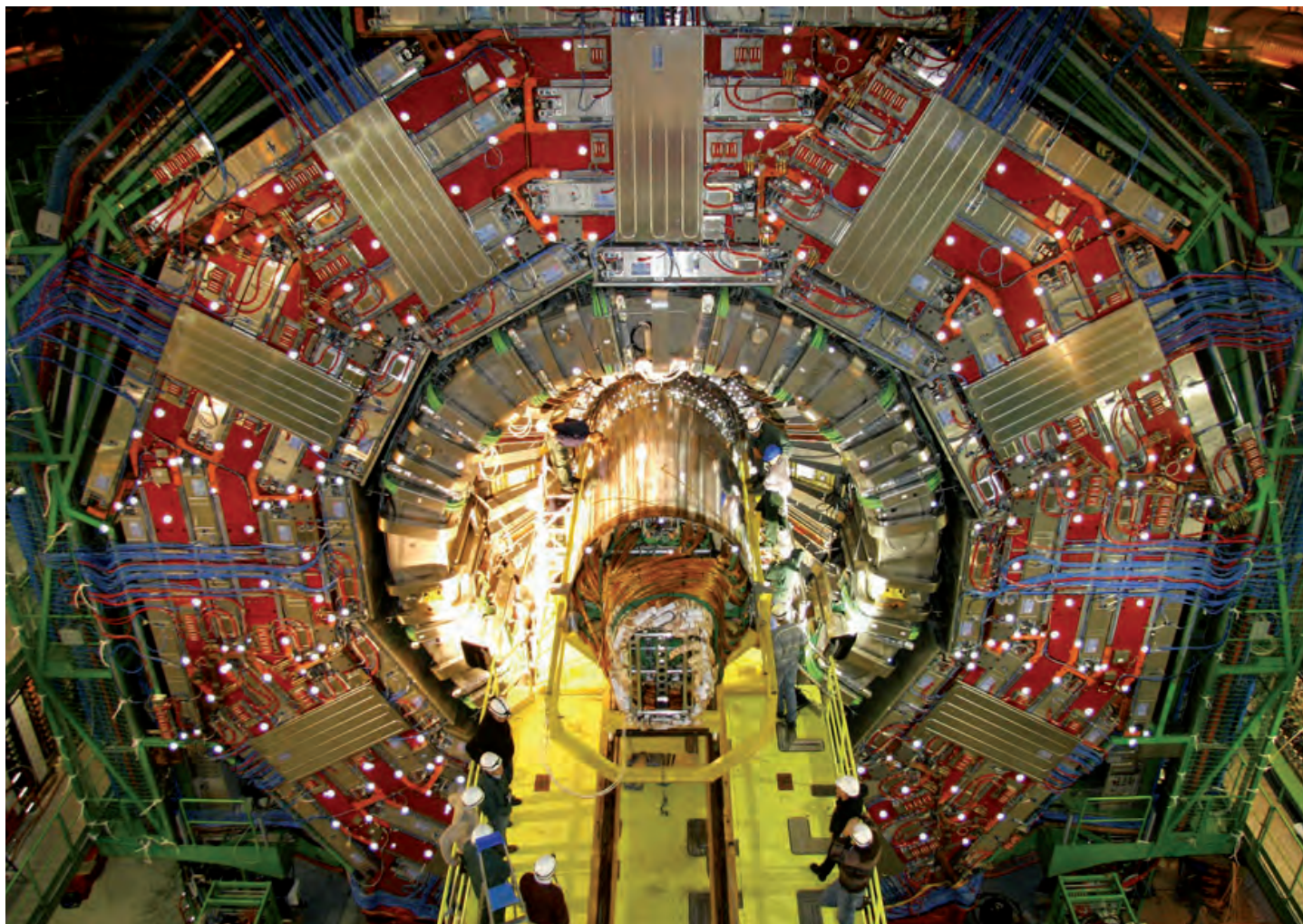
Installation of the world's largest silicon tracking detector in the CMS experiment. (Michael Hoch, ©CERN)
