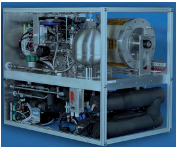
Front View of the OGA Equipment.
